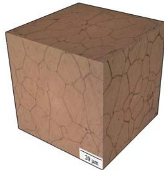
Fig. 2 SEM microstructures of solid-solution treated AZ80+2wt%Li Mg alloy.
